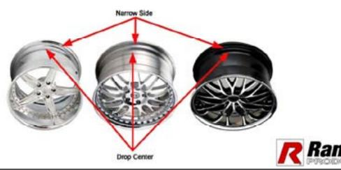
9. Place tire/wheel assembly on table top with mounting side up. (See Fig. 11.5)
