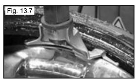
7. With the left side helper, press down on the tire near the right side assist roller to hold the tire in the drop center. (See Fig. 13.8)
