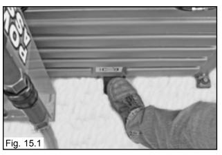
Tire Inflation – This is the activated position. With the inflation hose attached to the tire valve and the pedal depressed, line pressure is allowed to flow through the valve and into the tire for inflation. Tire pressure is indicated on the gauge in this position. (See Fig. 15.2-15.3)
