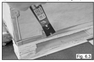
2. The entire wooden frame/box can be lifted off after prying the tabs/staples at the base of the crate. (See Fig 6.4)
