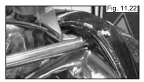
21. Depress the table top pedal to rotate the wheel clockwise. Leave the left hand helper in position opposite the demount head and allow it to follow the wheel rotation to assist the bead into drop center while demounting. Hold the tool bar down until demounting nears completion. (See Fig.11.23 - 11.25)
