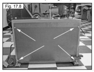
2. Loosen the four Motor mounting / adjusting bolts and nuts. (See Fig. 17.9)
