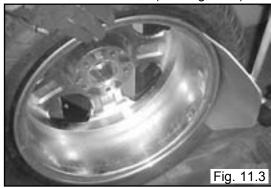
8. Determine the mounting side of the wheel. The mounting side is the narrow side of the drop center. The tire is removed for clarity. (See Fig. 11.4)
