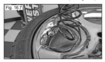
2. Hold tire up against upper edge of the wheel. Be sure tires top bead is over the bottom of the valve stem. (See Fig. 16.8)
