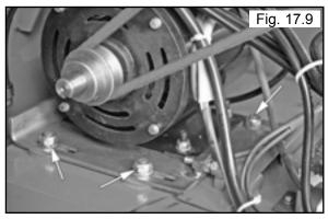
3. Inspect the Drive Belt for cracking and wear and replace as necessary. Adjust the Belt deflection to 3/8" - 1/2" using the Adjustment Bolt. Tighten all bolts when adjustment complete. (See Fig. 17.10)
