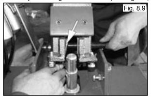
10. Be sure the Pin passes through the Safety Hook. Secure with the Snap Rings. (See Fig. 8.10)
