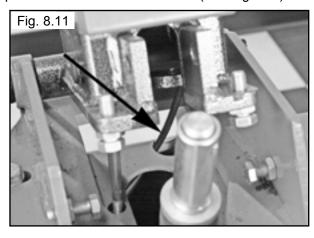
12. Align the Cylinder Shaft and cylinder pin and hole in the Tilt Tower and insert the Cylinder Pin. Secure the Cylinder Pin with the two Cotter Pins and bend Cotter pins. (See Fig 8.12)
