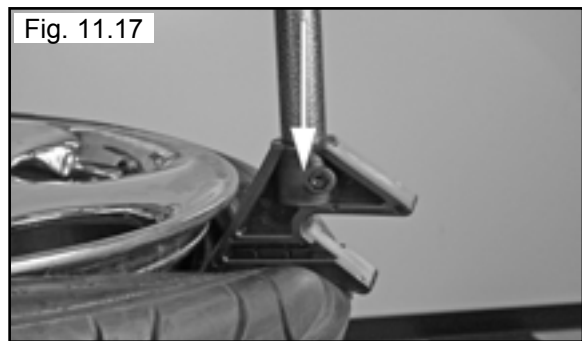
18. Power the left top helper down to force the tire bead into the drop the center of the wheel. (See Fig. 11.17-18)
