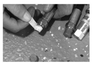
3. Install female quick-connect fitting onto threaded end.
