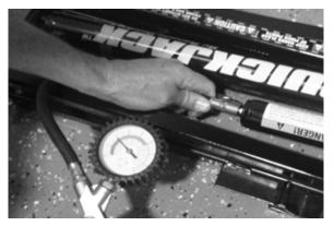
5. Press the air pressure gauge evenly onto the valve stem and record the reading given. If there is a hissing sound, the gauge is not tight or even enough for an accurate reading. **DO NOT EXCEED 50-PSI.**
