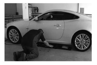
**TYPICAL JACKING POINTS** Always lift a vehicle according to the manufacturers recommended lifting points. Typical vehicle jacking points are illustrated below.
