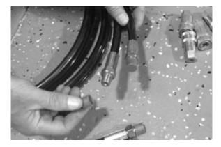
2. Wrap the threads with Teflon tape. When applying tape, wrap it three times in direction shown below.
