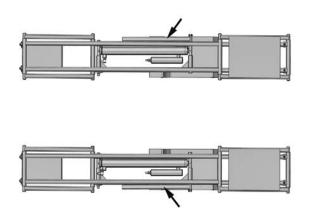
2. Check for proper tension on the safety lock bar retaining nuts. The safety lock bars should remain upright in the stowed position during normal use. They should be manually engaged when required.
