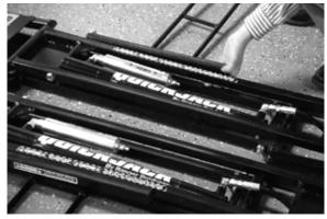
• **OUTSIDE IN**: In this method, the QuickJack frames are positioned wide enough for vehicle entry. Quick Frame Handles are typically not required. DO NOT drive over hydraulic hose. See below.
