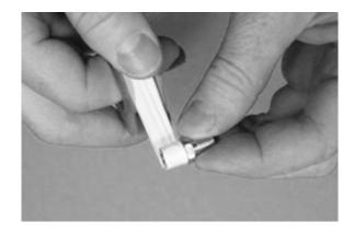
3. Carefully thread each air inflation valve into each air bottle cylinder as shown. NOTE: It is strongly recommended that valve cores be started by hand to minimize cross-threading.
