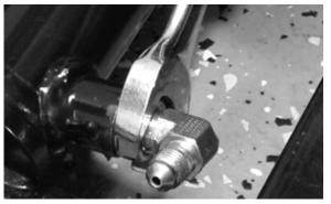
STEP 5 Installing Inflation Valves
