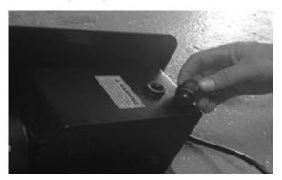
3. Fill the reservoir with approximately 2 quarts of automatic transmission fluid. Make sure the funnel used to fill the power unit oil reservoir is clean.
