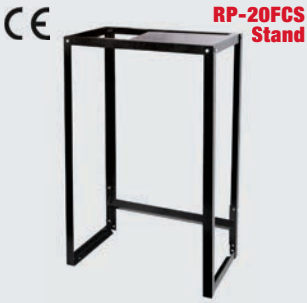
RP-20FCS Stand Capacity - 230 lbs. Unit Weight - 72 lbs. Dimensions - 27.75" x 42" x 17.75"
