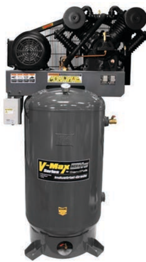
VMX-7580V-601 / 208-230 V / 60 Hz / 1 Ph Horsepower - 7.5 Hp Maximum CFM - 26.5 / 175 psi Tank - 300L / 80 Gal / Vertical
