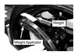
Pull the index arm out to the center plane position, the center WIDTH window will count down for you and display --0 when you have approached the correct position.
