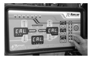
Press the **Down Arrow** below distance, then the **Up Arrow** below distance, LED lights will go blank.
