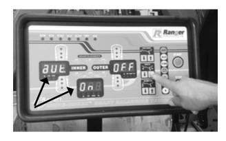
If the Width (middle screen) displays OFF, press the Width Arrow UP to change it to ON. If the middle screen displays ON, then the outer arm is already enabled.
