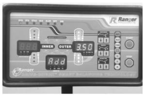
15. Replace weight at the 12 o'clock position on the OUTER side of wheel.
