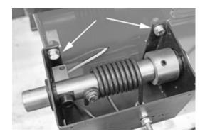
4. Slide the Hood Arm over the Hood Axle, align the holes in the Axle with the Allen bolts then secure in place using one Allen screw. Secure to shaft using a thick washer and Allen screw.
