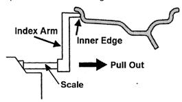
4. Read the offset measurement as displayed on the scale directly on top of index arm. Press the corresponding
