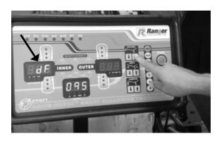
Press the **Distance UP Arrow**, four times, until **aut** shows on the inner window. (See below).
