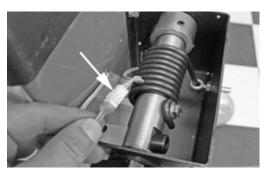
8. Tuck the wire into the Hood Switch Box and install Hood Switch Box Cover an tighten Allen bolts.
