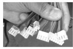
Be aware that CN4, CN8, and CN3 located on the bottom right (See image below), are color coded. Plug in these 3 pin connectors to their matching color terminals on the board.
