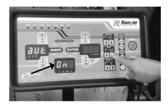
6. Press the **Distance Up Arrow** 3 times to advance to the original start-up balancer screen.
