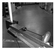
5. Run the wire coming off the gauge-arm thru the clips on the underside of the mounting arm.
