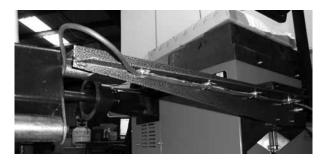
Attach the end of the wire to the connection on the back side of the balancer.
