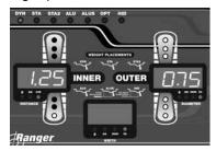
7. Attach the specified weight for the appropriate **PLANE** position at top-dead-center.
