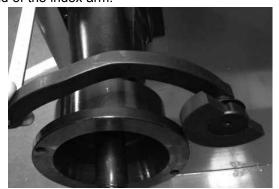
8. Pull the distance slide ruler out to 23.5cm / 235mm and rest the calibration disk against the flange.
