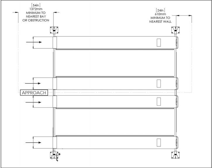
1. Lift Location: Use architects plan and Engineers automatic level (transit) when available to locate lift. The above shows clearances of a typical bay layout. Lift floor area should be level.
