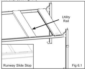
2. Place the other Inner Runway on top of the Crosstubes. Ensure that the Utility Rails is facing toward the Offside of the lift. Make sure the Runway is placed outside of the Runway Slide Stop. (See Fig. 6.2)
