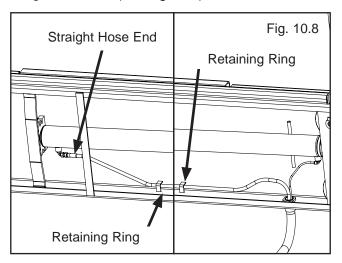
8. Connect the straight end of the Power Unit Hydraulic Line to the 90° Power Unit Fitting. Connect the Return Air Line to the 90° Air Fitting. There will be one air line hose left unconnected at this time. This air line hose will be used to activate the pneumatic safety locks on the next page. (See
