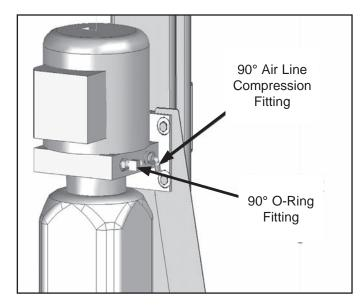
2. Remove the captive nut on the Compression Fitting. Insert the Plastic Air line through the alignment sleeve and into the end of the fitting until it bottoms out. Then tighten the nut on the fitting. (See Fig 10.3)
