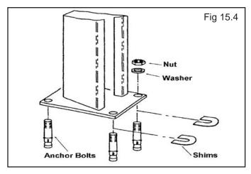
6. After any necessary shims are installed, tighten each nuts. IMPORTANT - If anchor bolts do not hold when torqued to required amount, concrete must replaced. Saw cut and remove 24" x 24" square area each column base then re-pour with reinforced 2500 concrete to a depth of six inches minimum, keying new concrete under existing floor. (See Fig. 15.5)
