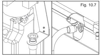
7. Connect the hydraulic hose and air line as shown below making sure the hydraulic hose passes through the retaining rings. MAKE SURE HOSES ARE KEPT CLEAR OF CABLES. There will be one air line hose left unconnected in this step. This air line will be used to activate the pneumatic safety locks in the next step. See page 19 for Compression Fitting instructions. (See Fig. 10.8)
