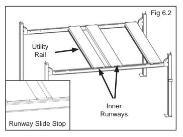
3. Position the Offside Runway on top of the Cross Tubes with the utility rail towards the center. Align the holes in the Runway with the holes on both ends of the Cross Tubes and bolt together. Bolt down the Offside Runway using the same procedure as for the Powerside Runway. (See Fig 6.3)
