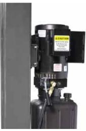
An air supply (minimum 30 psi / 3 CFM) is required for the safetylock mechanisms to disengage. It is solely the responsibility of the end-user to provide, install and maintain the air supply.
