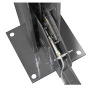
An air supply (minimum 30 psi / 3 CFM) is required for the safety-lock mechanisms to disengage. It is solely the responsibility of the end-user to provide, install and maintain the air supply.
