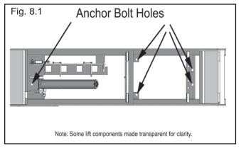
3. Using a 3/4" concrete bit, drill five holes on each pad 5" deep using the holes in the frame as a guide. (See Fig 8.2)
