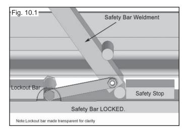
4. Check all MAIN SAFETY LOCKS to make sure they move freely and fall back to the lock position when released. Lubricate all SAFETY PIVOT points with WD-40 or equal.
