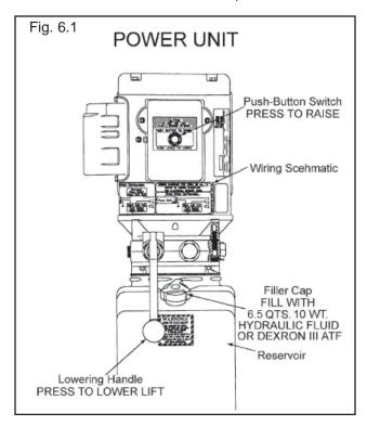
3. The standard power unit for your lift is 110 volt, 60HZ, single phase. All wiring must be performed by a certified electrician only. SEE WIRING INSTRUCTIONS AFFIXED TO MOTOR FOR PROPER WIRING INSTRUCTIONS.
