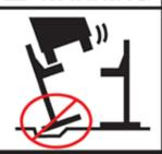
Locate lift on firm, level surface, preferably concrete.
