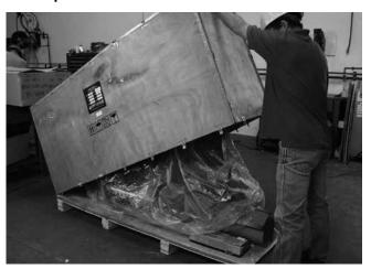
Remove the Control Pod, Sliding Carriage. Grease Gun and Tire Irons from the pallet and set aside.
