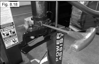
4. Once the plastic demount head has been removed you can place the metal demount head in place. Make sure the top of the demount head is is pressed firmly against the plastic hex shaft spacer and tighten both the allen set screws and the bottom hex nut. (See Fig. 8.19)
