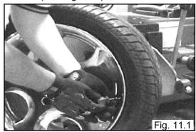
2. The clamps on the table top may extend beyond the table top itself. To avoid damaging the clamps and/or wheel, move the clamps to their full inward position before positioning a tire for bead loosening.
