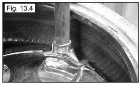
5. Manually force the tire down into the drop center of the wheel directly across from the mount head to reduce the tensional force on the bead. Depress the table top pedal and rotate the wheel to mount the lower bead. Rotate the table top until the lower bead is fully mounted.
