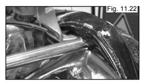
21. Depress the table top pedal to rotate the wheel clockwise. Leave the right hand helper in position opposite the demount head and allow it to follow the wheel rotation to assist the bead into drop center while demounting. Hold the tool bar down until demounting nears completion. (See Fig.11.23 - 11.25)
