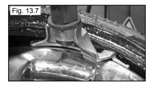
7. With the right side helper, press down on the tire near the right side assist roller to hold the tire in the drop center. (See Fig. 13.8)
