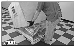
3. Carefully cut the plastic wrapping and remove.
