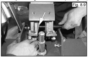
10. Be sure the Pin passes through the Safety Hook. Secure with the Snap Rings. (See Fig. 8.10)
