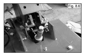
7. Insert the man Pivot Pin though the holes in the Tilt Tower Base and Tilt Tower and secure the Nyloc Nuts. (See Fig. 8.7)
