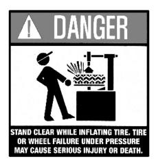
1. Once tire pressure is indicated on the air gauge (inflation pedal depressed, continue to inject air into the tire in short intervals. Check the pressure frequently. Stand back during bead seat. Keep hands, arms, and entire body away from tire during this procedure. Tire beads should move outward and "pop" into their bead seat position as pressure inside the tire increases. If this does not happen, a problem exists. Investigate carefully. (See Fig. 16.12)
