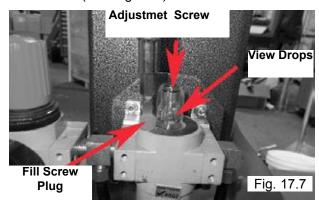
(Either reservoir may be removed for cleaning by turning the reservoir counter-clockwise and pulling down.)
