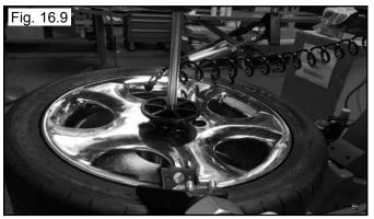
The blast of air from the valve will expand tire and seal the beads. (See Fig. 16.10)
