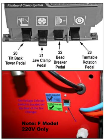
Note: The parts and procedures shown in this manual include optional equipment that may not be included on the model of Tire Changer you are using.
