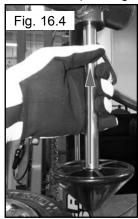
2. Make sure the restraint tool is centered in the center hub of the wheel then press down on the left hand control valve. (See Fig.16.5-16.6)
