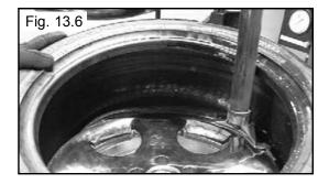
6. For the top bead, rotate the table top until the valve stem is directly across from the mount head. Lift the upper bead above the left "duckbill" side of the mount/demount head and below the right front knob. (See Fig. 13.7)
