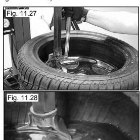
24. Depress the table top pedal to rotate the wheel. The demount head will guide the bead up and over the edge of the wheel. Continue rotation until the lower bead is de-mounted. The helper disk should be removed during rotation. Swing the disc out of the way to complete de-mounting. (See Fig. 11.29)
