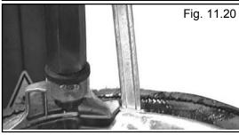
20. Push the tool bar down toward the wheel to lift the tire bead up and over the right -side knob portion of the demount head. Hold the tool bar in this position. (See Fig. 11.21 - 11.22)
