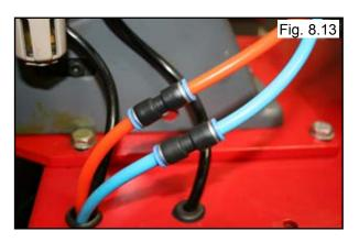
16. Connect the Air Line from the Tilt Back Tower to the Tee Fitting located Inside the Rear of the Cabinet. (See Fig 8.15)
